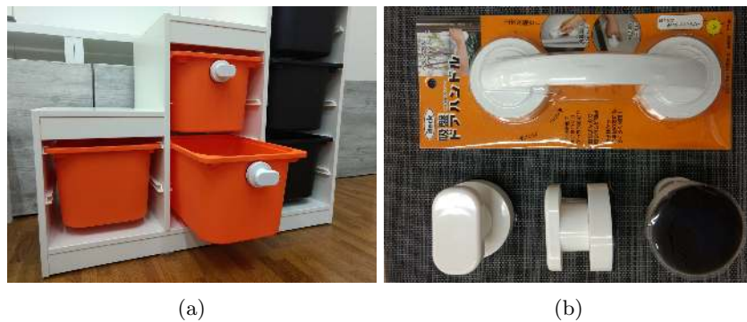
Figure 4: a) Stairs-like drawer. The drawer will be as it is (left drawer) or it might have a handle and/or be opened under team request (middle drawers). b) Several views of the easy-to-manipulate handles in two different sizes, namely large (top part of the image) and short (bottom part).
